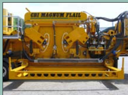
Hydraulic debris-removal conveying ram with support frame to ensure perfect alignment
