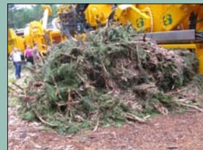
Bark discharges on opposite side of chip discharge. Designed to push bark/debris far from discharge chute
