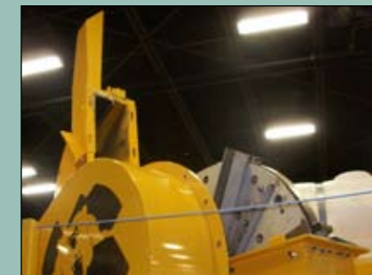
Complete chipper hood opens hydraulically for easier service and exposes 180° of disc. Bolt-in liners throughout
