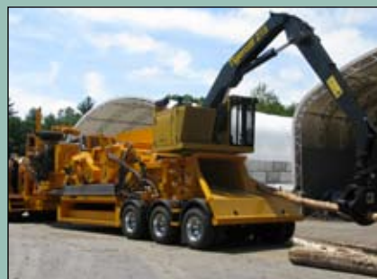
Independent, fully-equipped Tigercat loader with remote control for complete system
