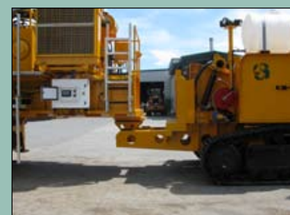
Direct feed from Flail to Disc Chipper. No extra loader required. Camera monitored so operator knows debarking efficiency level
