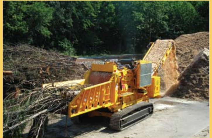
An additional foot has been added to the feed table specifically for high-volume applications.
