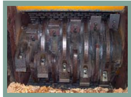
Solid Steel Rotor with optional Brute Package and bolt-on strikers. Perfect for contaminated C&D, railroad ties, telephone poles, etc.
