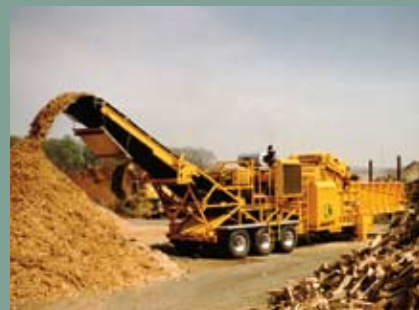
Construction wood to high-quality fuel
